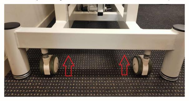
The next step is to pull the locking lever up and down quick approx. 5 times. Then push the lever back down to lock the wheels. This will re-engage the wheel system.
