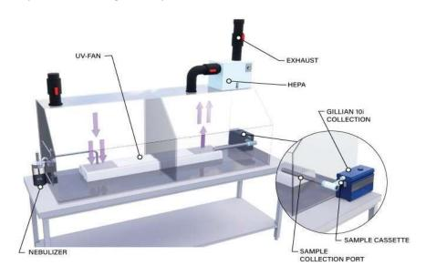
units were injected into the airflow and samples were taken after the air had passed through the purifier, to evaluate the presence or absence of active viruses still capable of being "infectious".
