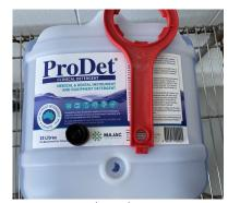
Unscrew the "bung" using the spanner or similar tool, by turning anti-clock wise
