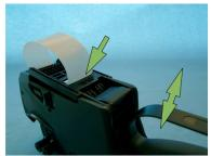
In case of a rarely misprint one can adjust the printing position manually by loosen this screw and adjust the slide a bit to the back or front. After adjusting one should tight the screw again. The screw can be reached through the backing material.
