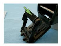
The ink roller is now easily accessible and can be easily replaced by a new one. Please always use genuine parts in order to prevent clogging of the characters and misprints or smearing as a result.
