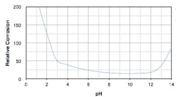
This chart shows the relative corrosion of iron at various pH values in oxygen free solutions. It shows that the corrosion of iron is lowest in the pH range 7 to12. This is why in many industrial situations water is maintained in an alkaline pH in order to minimize the corrosion of iron and steel.<sup>1</sup>
