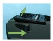
To be able to load labels into the label gun one should open the bottom of the label gun by pushing both levers at the side backwards. The bottom of the label gun will open itself after which one can push the bottom backwards to have a full access to place the label roll into the gun.
