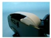
Unroll the label roll partly and take off about 8 labels. Push the roll into the label gun as per picture. The labels are pointing toward the top of the label gun.
