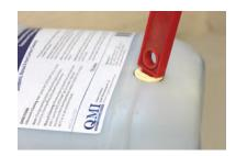
**6.** Unscrew the "bung" using the spanner or similar tool by turning anticlockwise.
