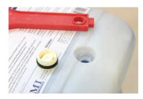
7. When the "bung" is removed check that there is a hole drilled under the bung.
